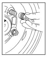
Put the wheel nuts back on with the rounded end of the nuts toward the wheel. Tighten each nut by hand until the wheel is held against the hub.
